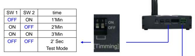
Test mode:== put "OFF" position [Active AC output power 2 seconds then Stop].
